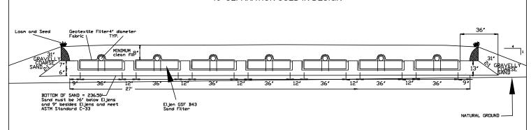
NOTE: REMOVE VEGETATION AND SCARIFY ORIGINAL SOIL UNDER ENTIRE FILL AREA NOTE: THOROGHLY MIX CLEAN, COARSE, SHARP SAND INTO TOP 4 INCHES OF ORIGINAL SOIL TO CREATE A TRANSITION ZONE
