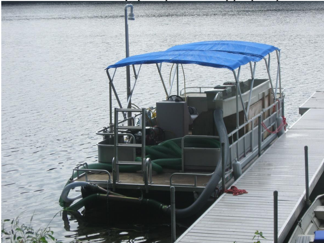
CPIA DASH Boat-1990 Sea Nymph 50hp outboard 23hp pump/compressor
