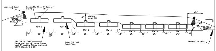
NOTE: REMOVE VEGETATION AND SCARIFY ORIGINAL SOIL UNDER ENTIRE FILL AREA NOTE: THOROGHLY MIX CLEAN, COARSE, SHARP SAND INTO TOP 4 INCHES OF ORIGINAL SOIL
