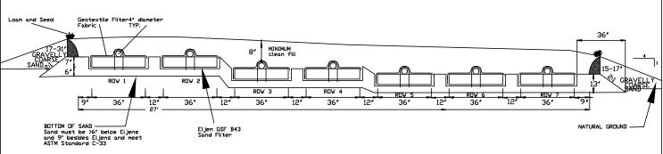
NOTE: REMOVE VEGETATION AND SCARIFY ORIGINAL SOIL UNDER ENTIRE FILL AREA NOTE: THOROGHLY MIX CLEAN, COARSE, SHARP SAND INTO TOP 4 INCHES OF ORIGINAL SOIL TO CREATE A TRANSITION ZONE
