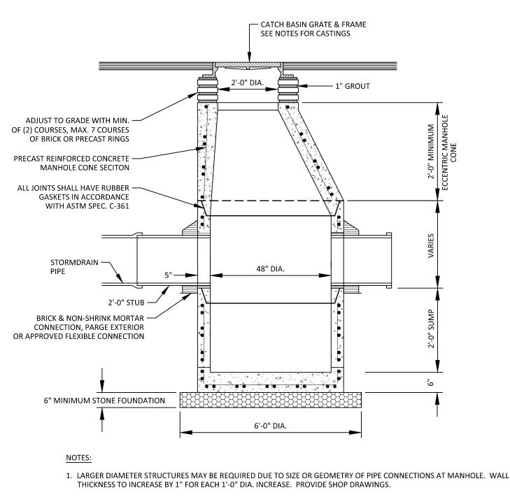
2. DRAINAGE STRUCTURES TO BE DESIGNED FOR H-20 LOADING.
