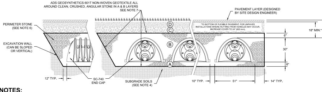
1. THE LISTED AASHTO DESIGNATIONS ARE FOR GRADATIONS ONLY. THE STONE MUST ALSO BE CLEAN, CRUSHED, ANGULAR. FOR EXAMPLE, A SPECIFICATION FOR #4 STONE WOULD STATE: "CLEAN, CRUSHED,
