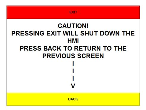
**SET DATE AND TIME:** On the SYSTEM SETUP SCREEN select the hidden button in the upper left hand corner. It will ask you if you want to EXIT. To reset the DATE and TIME select EXIT.
