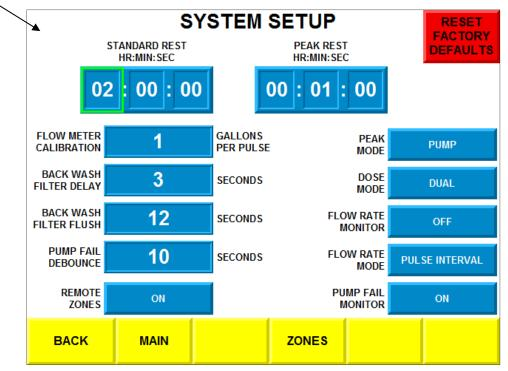
**STANDARD / PEAK REST:** Enter the desired rest time between the start of cycles.
