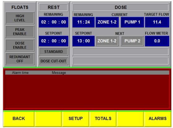
**FLOATS:** Gray background indicates that the float switch is not activated (down position). Green background indicates the float is activated.
